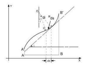
Consider a beam AB which is initially straight and horizontal when unloaded. If under the action of loads the beam deflect to a position A'B' under load or infact we say that the axis of the beam bends to a shape A'B'. It is customary to call A'B' the curved axis of the beam as the elastic line or deflection curve.
