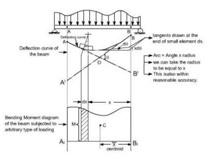
Refer to the figure shown above consider AB to be any portion of the elastic line of the loaded beam and  $A_1B_1$  is its corresponding bending moment diagram.
