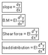
**Methods for finding the deflection:** The deflection of the loaded beam can be obtained various methods. The one of the method for finding the deflection of the beam is the direct integration method, i.e. the method using the differential equation which we have derived.
