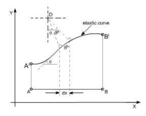
It may be noted that dq is an angle subtended by an arc element ds and M is the bending moment to which this element is subjected.
