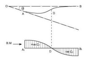
Then, adequate precaution must be exercised in using the above theorem. In such a case B. M diagram gets divide into two portions +ve and –ve portions with centroids  $C_1$  and  $C_2$ . Then to find an angle q between the tangents the points A and B
