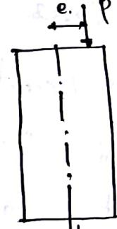
1. The load  $P$  is applied along the line of axis of the column, two equal & opposite force  $P$  are acting now on the column.
