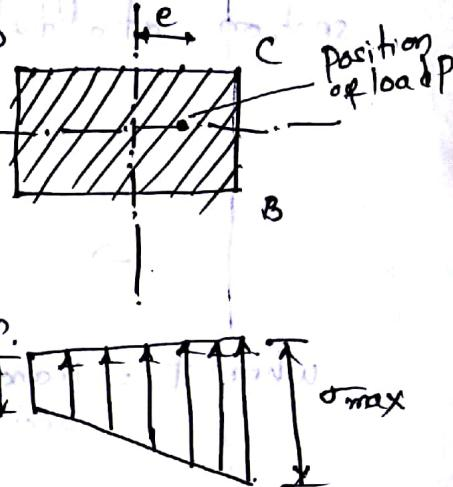
These stresses are shown in fig. The resultant stress along the width of the column will vary by a straight line law.
