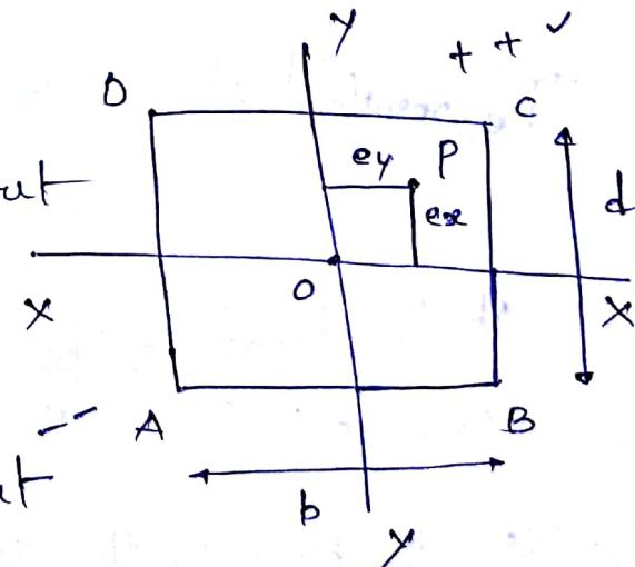
Now the eccentric load is equivalent to a central load  $P$ , together with a bending moment  $P \times e_y$  about  $y-y$  & a bending moment  $P \times e_x$  about  $x-x$
