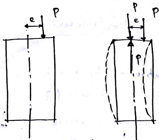
Hence an eccentric load will produce a direct stress as well as a bending stress. By adding these two stresses algebraically, a single resultant stress can be obtained algebraically.
