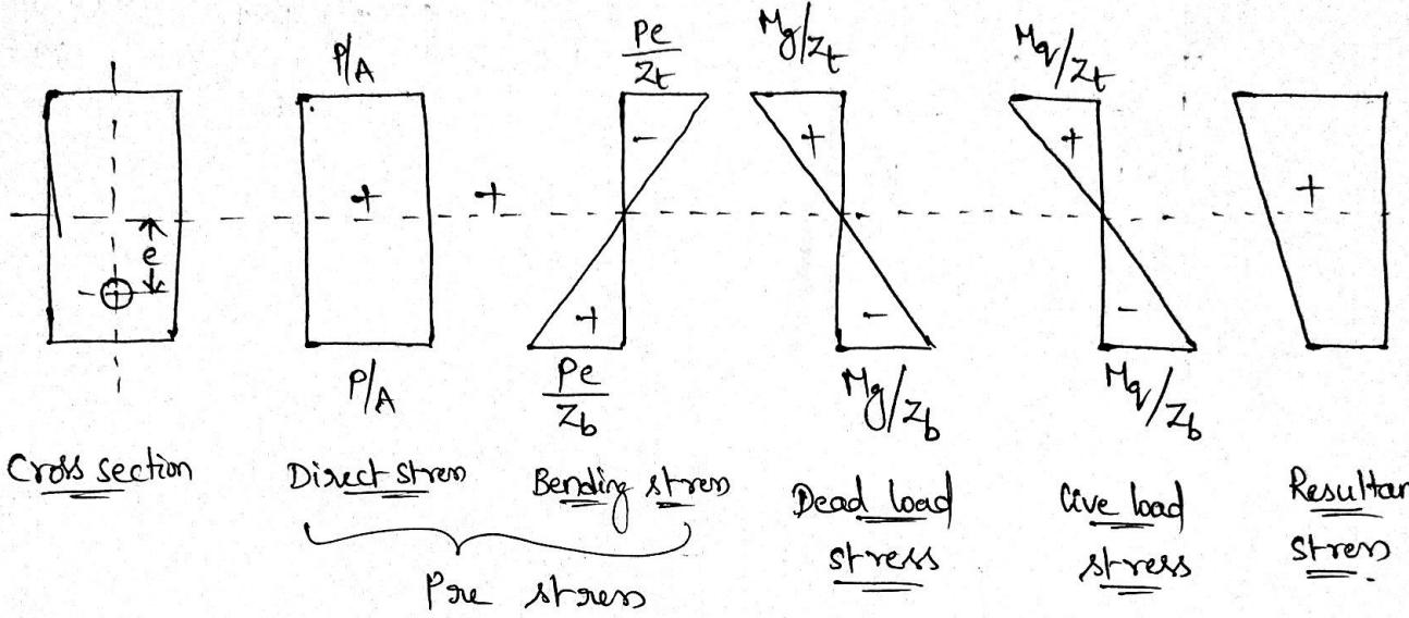
$$\text{Resultant stress at top} = \frac{P}{A} - \frac{Pe}{Zt} + \frac{Mg}{Zt} + \frac{Mq}{Zt}$$
