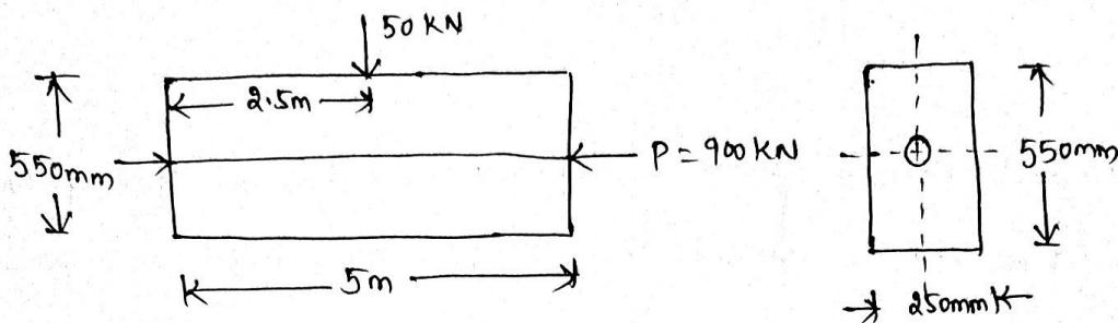
$$\text{Gross c/s area, } A = 0.25 \times 0.550 = 137.5 \times 10^3 \text{ mm}^2$$
