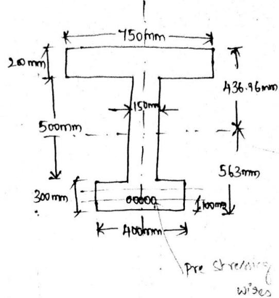
$$(ii) \text{ at the bottom fibre} = \frac{Pe}{Z_b} = \frac{2003.02 \times 10^3 \times 463.04}{7.187 \times 10^7} \leftarrow (563.04 - 100)$$
