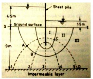
The no. of flow channels,  $n_f = 3$ The no of drops,  $n_d = 6$ Diff. of u/s head and d/s head =4.5-1.5 = 3 m Loss of head per drop = 3/6 = 0.5 m
