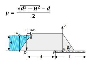
Select the base of the dam and directrix as x and z-axes.
