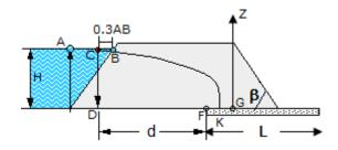
6. Upstream Correction: Sketch the section BE such that it is normal to the upstream sloping surface (i.e. equipotential line). BEK is the phreatic line (top flow line)
