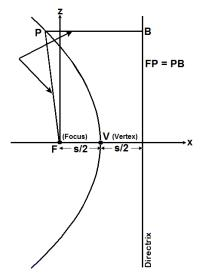
Every point on the parabola is equidistant from the focus and directrix.
