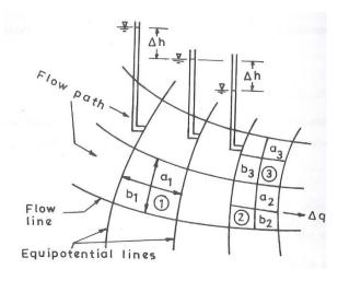
Let  $\Delta q_1$ ,  $\Delta q_2$ , and  $\Delta q_3$  be the rate of flow through fields 1, 2 and 3, respectively, and  $\Delta h_1$ ,  $\Delta h_2$ , and  $\Delta h_3$  be the head loss across the fields 1, 2 and 3.
