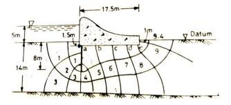
Elevation head for points at upstream end of toe, a, b, c, d, e = -1.5m (-ve sign as elevation is measures below datum)
