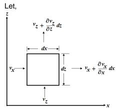
Velocity at the inlet face in the horizontal direction =  $v_x$ Velocity at the inlet face in the vertical direction =  $v_z$ Velocity at the outlet face in the horizontal direction =  $v_x + \frac{\partial v_x}{\partial x} dx$
