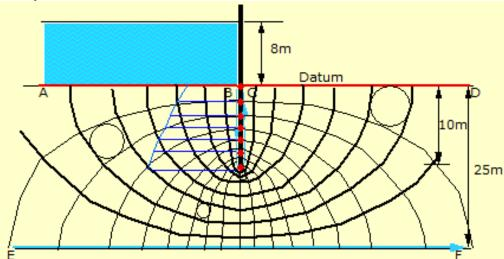
Total number of drops = 18  $\therefore$  8m head is lost in 18 drops Head loss per drop = 8/18 = 0.44 m
