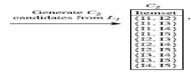
4. The transactions in D are scanned and the support count of each candidate itemset in C2 is accumulated.
