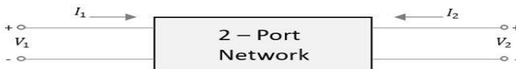
Structure of a two port network
