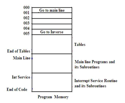
When we deal with tables, they are assigned to addresses in the range H'005 - H'0FF' because for most of the applications this space is sufficient. The main line program begins after the tables.
