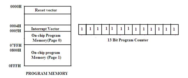
Two addresses in the program memory address space are treated in a special way by the CPU. The first address H' 000' being a go to mainline instruction the second special address, H' 004' being a 'go to in service' instruction can be assigned to this address to make the CPU to jump to the beginning of the Interrupt Service routine located elsewhere in the memory space.
