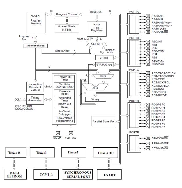
**Block diagram of PIC 16F87X Microcontroller**
