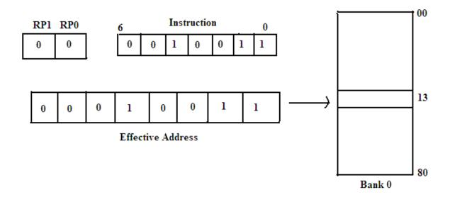
The above diagram explains the method of accessing register file address 13H by direct addressing method.
