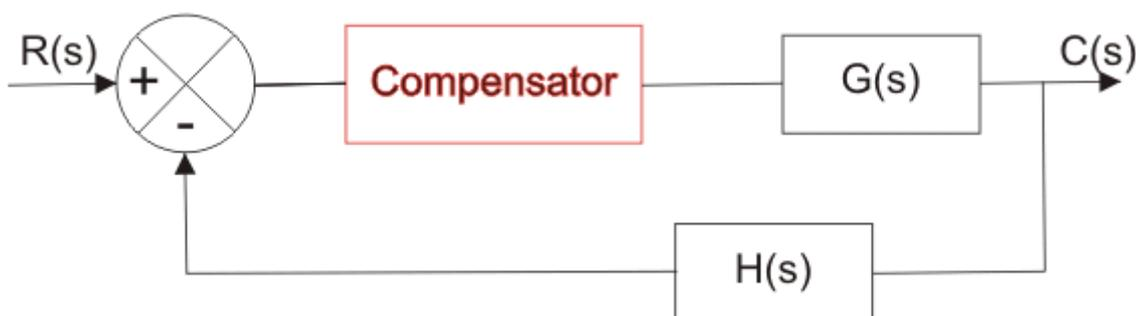
Fig 1.7: Series Compensator
