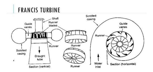
A reaction turbine develops power partly due to the velocity of water and partly due to the difference in pressure acting on the front and back of the runner buckets.
