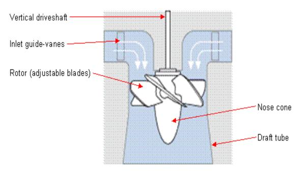
A Kaplan turbine is a propeller' turbine with adjustable blades, the advantage of adjustable blades being that a Kaplan turbine operates at high efficiency even under part load conditions.
