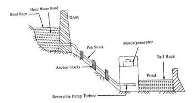
Pumped storage plants are a special type of power plants which work as ordinary hydro power plants for part of the time and when such plants are not producing power, they can be used as pumping stations which pump water from tail race to the head race.
