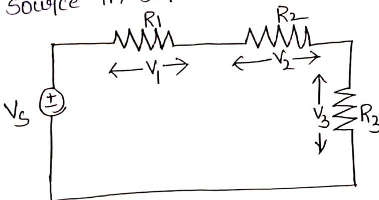
Let  $V_s$  is the source voltage and  $V_1, V_2, V_3$  are the voltage drops.
