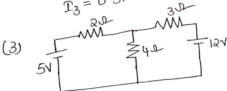
calculate the current flowing through 4Ω resistor.
