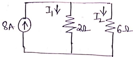
⑧ calculate  $I_1, I_2$  from the given circuit
