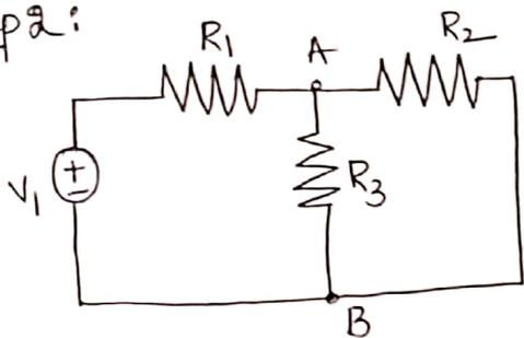
Now  $V_1$  source is acting independently and  $V_2$  is replaced by short circuit. Obtain current through AB branch. ( $I'_{AB}$ )
