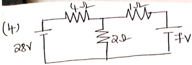
Calculate power loss in each element.
