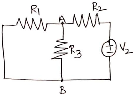
Now consider  $V_2$  alone and  $V_1$  is replaced by short circuit. Obtain current through AB branch. ( $I''_{AB}$ )
