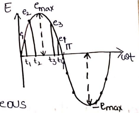
Ex:  $e_1, e_2, e_3$  &  $e_4$  are instantaneous values of alternating Emf at the instants  $t_1, t_2, t_3$  &  $t_4$  respectively
