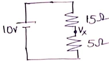
⑥ calculate the voltage  $v_5$  from the given circuit
