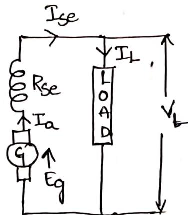
The voltage equation is  $E_g = V_L + I_a R_a + I_{se} R_{se} + V_b$
