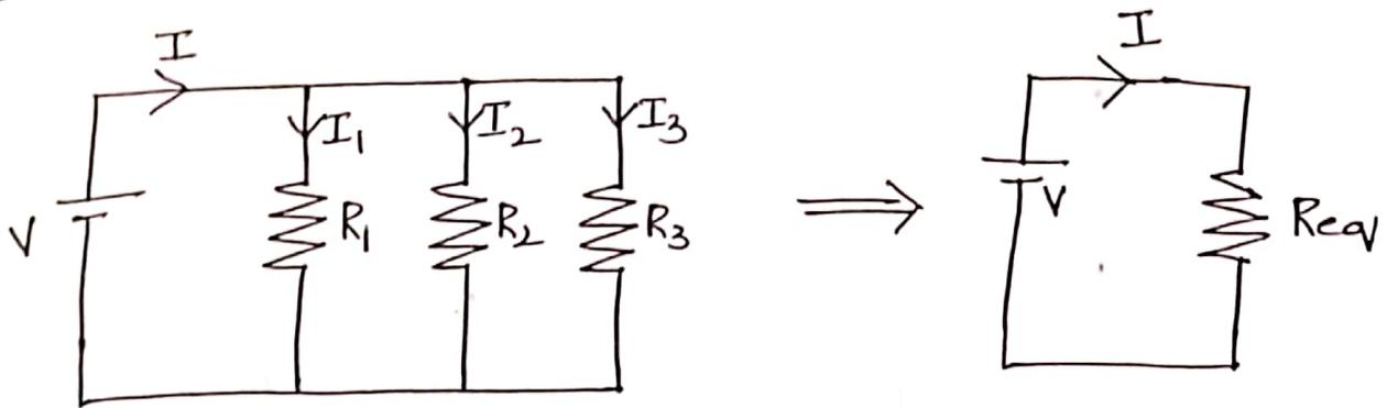
Consider the circuit,  $R_1, R_2, R_3$  are connected in parallel. This combination is connected across a source voltage  $V$ . The voltage across the two ends of each resistance  $R_1, R_2, R_3$  is same and equal to the supply voltage  $V$ , and current is dividing at principle node.
