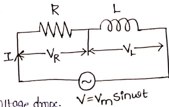
Voltage drop due to resistor  $V_R = IR$
