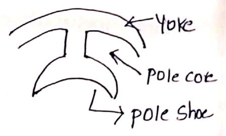
② pole shoe: pole shoe enlarges the area of armature core to come across the flux which is necessary to produce large EMF. It is made up of cast iron (or) steel, laminated construction.
