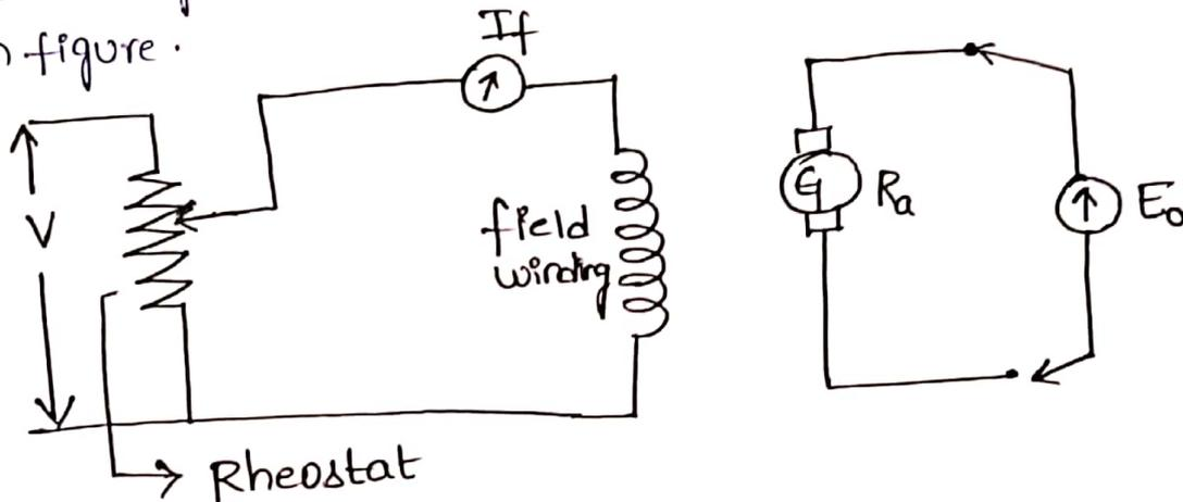
The Rheostat as a potential divider is used to control the field current and the flux. It is varied from zero and is measured on ammeter connected.
