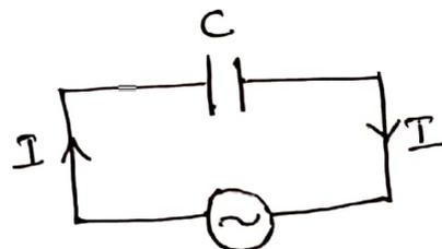
Then the response flowing through capacitor is  $V = V_m \sin \omega t$
