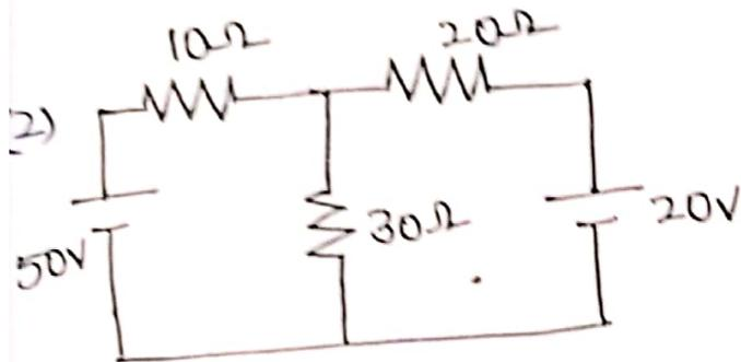
Using superposition theorem
