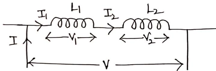
If two inductors  $L_1$  and  $L_2$  are connected in series as shown in the fig,
