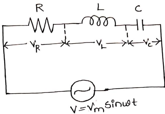
The AC supply is given by  $V = V_m \sin \omega t$ .
