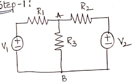
Calculate the current in branch A-B of the network using Superposition theorem.  $I_{AB}$
