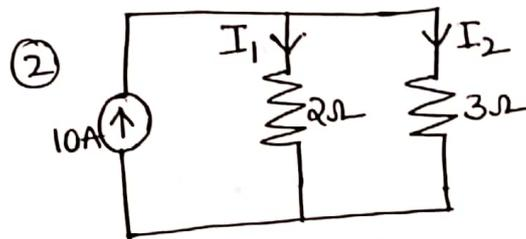
Calculate  $I_1, I_2$  by using current division rule also find voltage drop across the elements.
