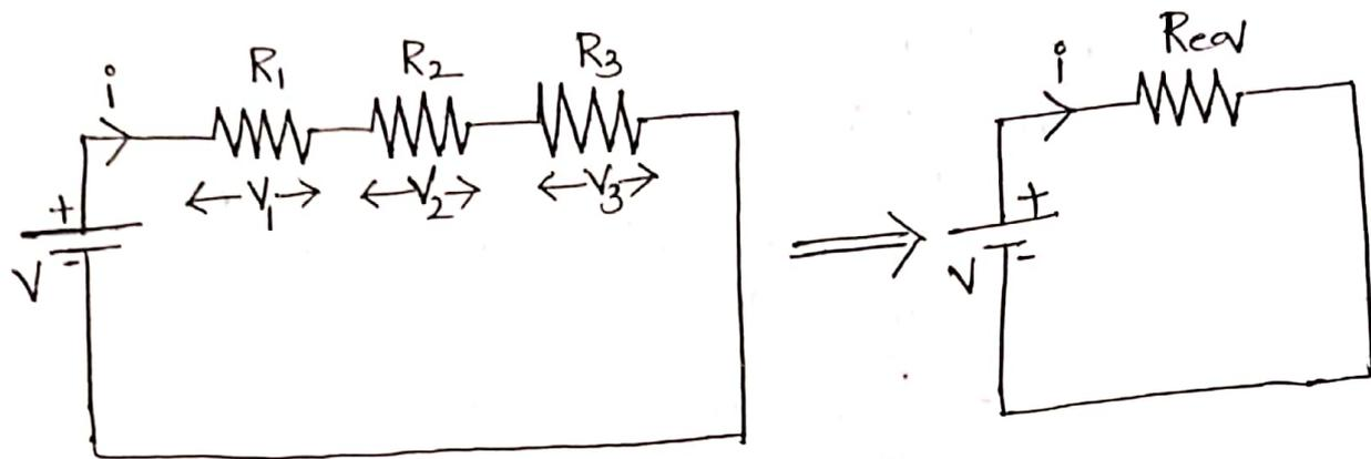
Consider the circuit, where  $R_1, R_2, R_3$  are connected in series. This combination is connected across a source voltage 'V'.
