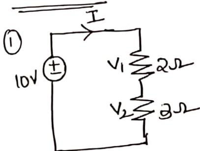
Calculate  $V_1$  &  $V_2$  by voltage division rule
