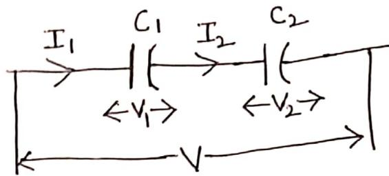
If two capacitors  $C_1$  and  $C_2$  are connected in series as shown in the fig
