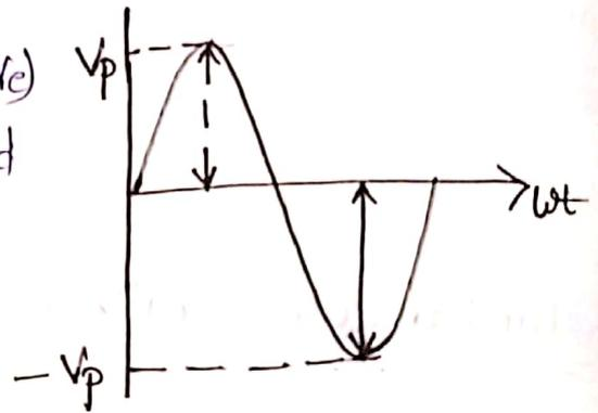
\* The peak-to-peak value of sine wave-form is the value from +ve peak to -ve peak. denoted by  $V_{p-p}$
