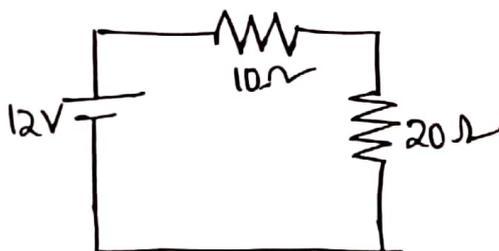
④ calculate  $v_1, v_2$  in the following circuit
