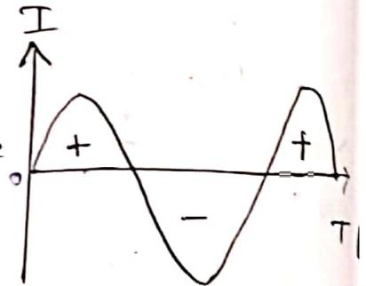
Such change in magnitude and direction is measured in terms of cycles. Each cycle of AC consists of two half cycles namely positive cycle and negative cycle. Current increases in magnitude, in one particular direction, attains maximum and starts decreasing, passing through zero, it increases in opposite direction and behaves similarly as shown in the figure.
