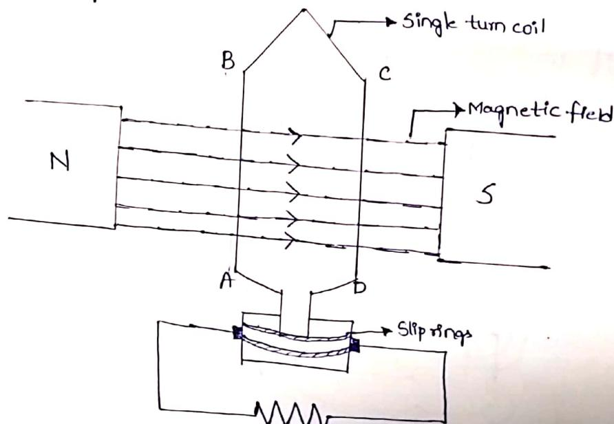
Let us consider a single turn coil (A, B, C, D) is placed in a magnetic field as shown in the figure. The conductor ends are connected to two slip rings which are mounted on shaft. Two stationary brushes (B<sub>1</sub> & B<sub>2</sub>) are mounted on slip rings which collect the current and passes it to external circuit.
