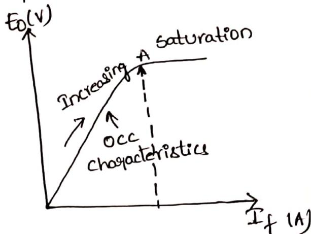
As  $I_f$  is varied, then  $\phi$  changes and hence induced emf  $E_0$  also varies. It is measured on Voltmeter connected across armature.
