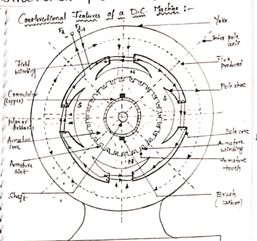
A DC machine mainly consists of two parts such as
