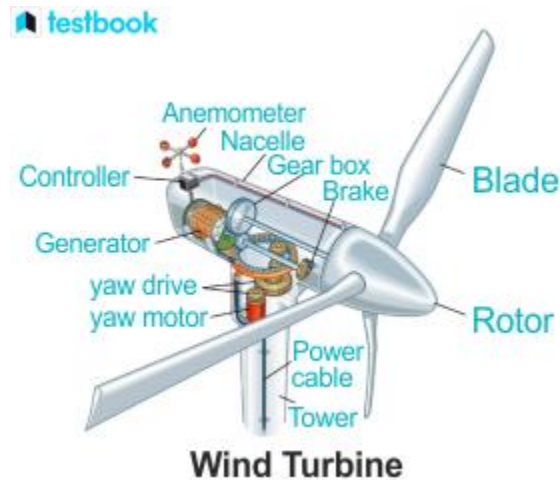
Fig 4: Construction and Working of Windmill
