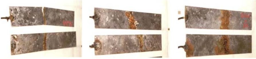
Figure 8.5 Visual observation of the corrosive attack on bare steel plates embedded in reference natural-aggregate concrete N0.3 (left), in recycled-aggregate concrete R0.3 (middle), and high-fly-ash-volume concrete N0.3F (right).
