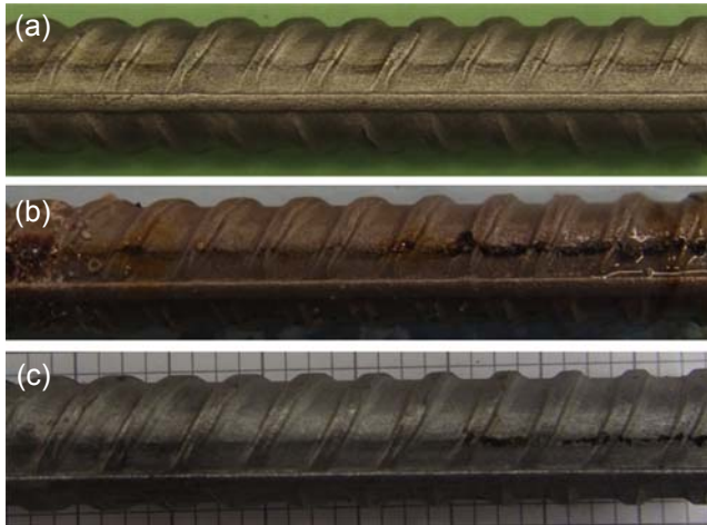
Figure 4.11 Corrosion of 316LN along a processing defect: (a) as-received bar; (b) after exposure to pore solution with increasing chloride content up to 16%; and (c) after pickling in inhibited acid (Bandura, 2015).
