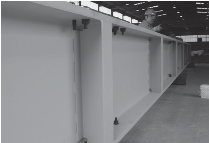
This beam is to be subjected to heavy concentrated loads. Full depth web stiffeners are used to prevent web crippling and to keep the top flange from twisting or warping at the load. (Courtesy of CMC South Carolina Steel.)
