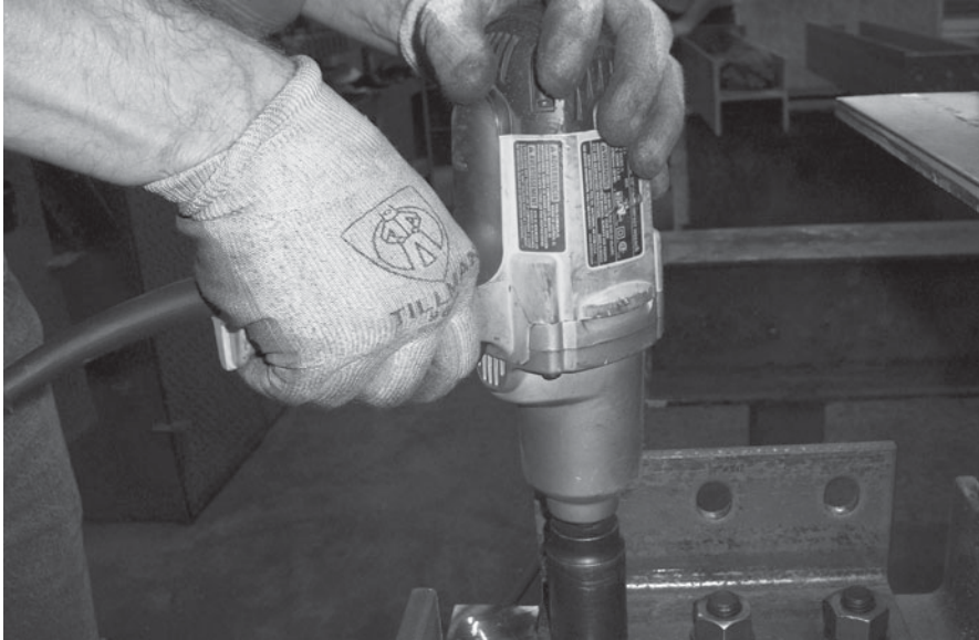
An impact wrench used to tighten bolts to either a snug-tight or a fully tensioned condition. It may be electric, such as this one, or it may be pneumatic. (Courtesy of CMC South Carolina Steel.)
