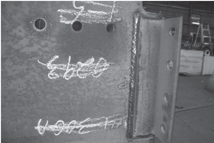
A typical framing angle shop-welded to a beam. It will be field-bolted to another member. (Courtesy of CMC South Carolina Steel.)
