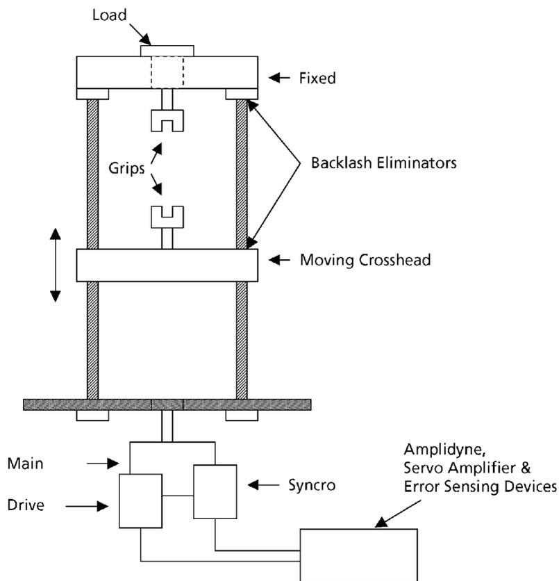
**Figure 6.13** Achematic of an electromechanical twin-screw tensile test machine
