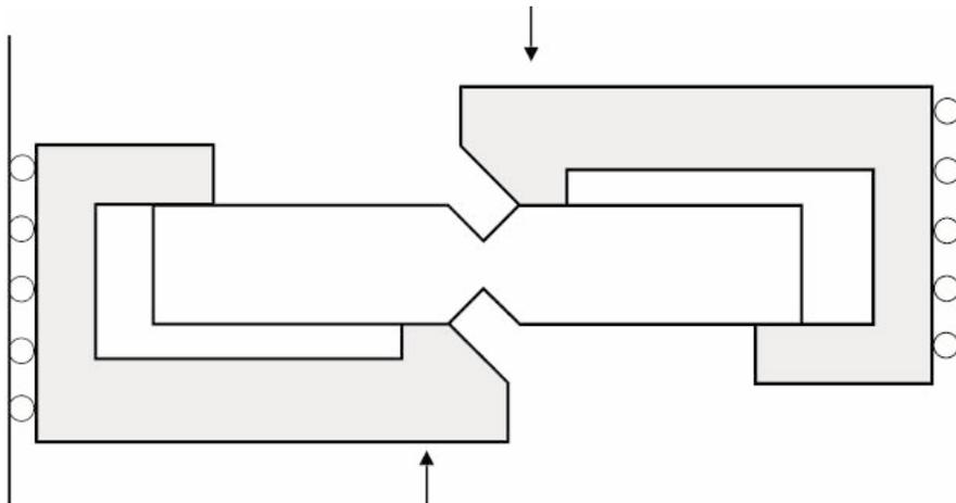
Figure 8.6 Loading arrangement for Iosipescu test piece
