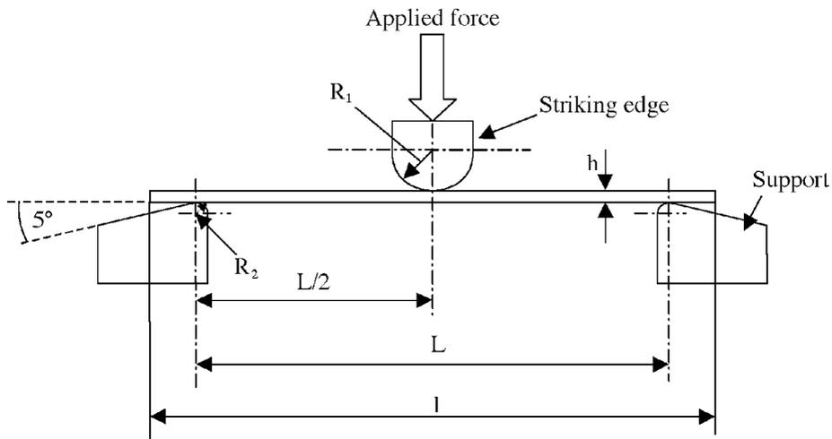
Figure 9.3 ISO 178 test arrangement
