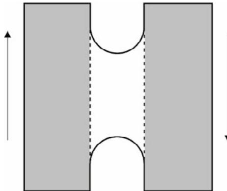
Figure 8.5 Shear Test Piece after Hedner [14]
