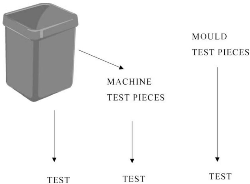
Figure 1.4 Choices for impact testing of a bucket
