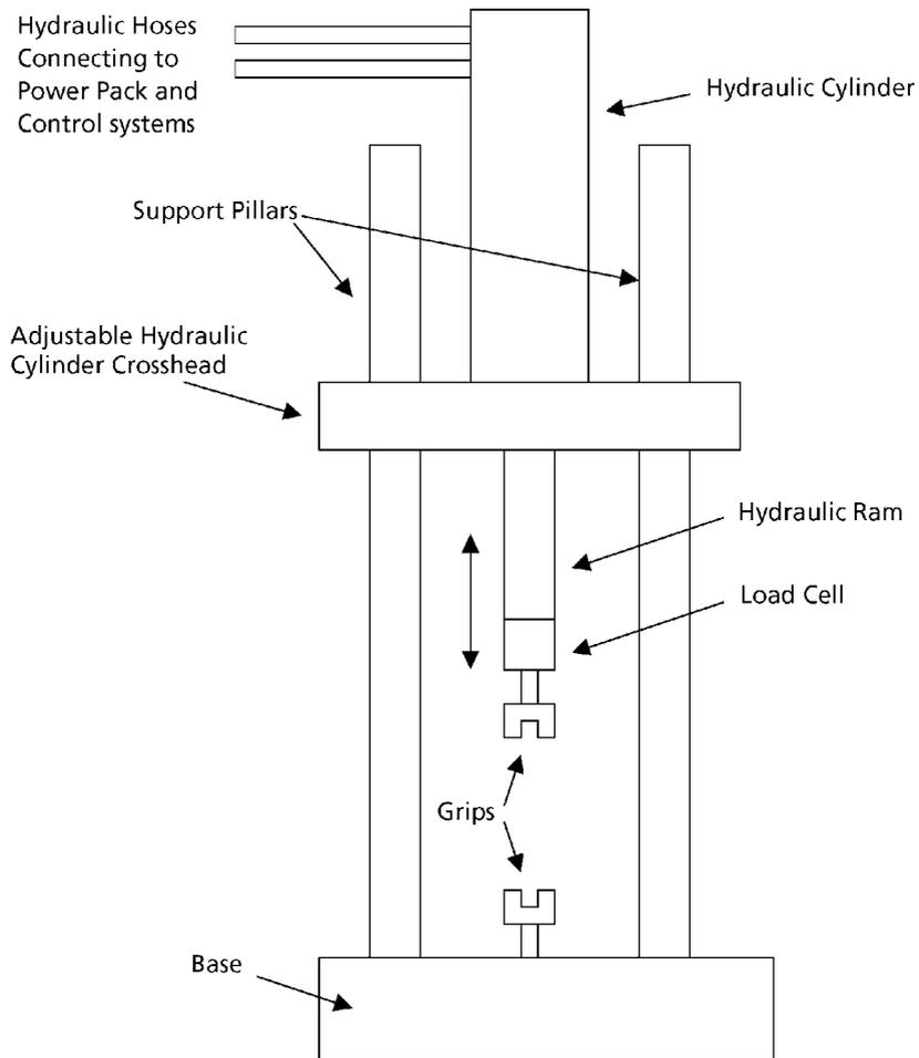
Figure 6.14 Schematic of a servohydraulic tensile test machine
