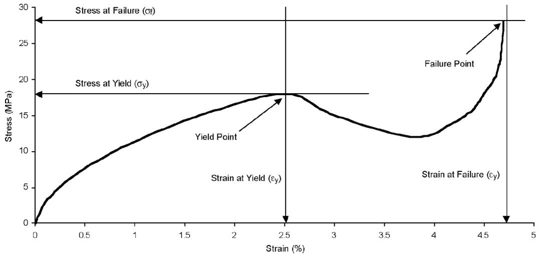
**Figure 6.6** Typical non-linear stress *versus* strain characteristic of tough thermoplastic with a failure stress greater than the yield point
