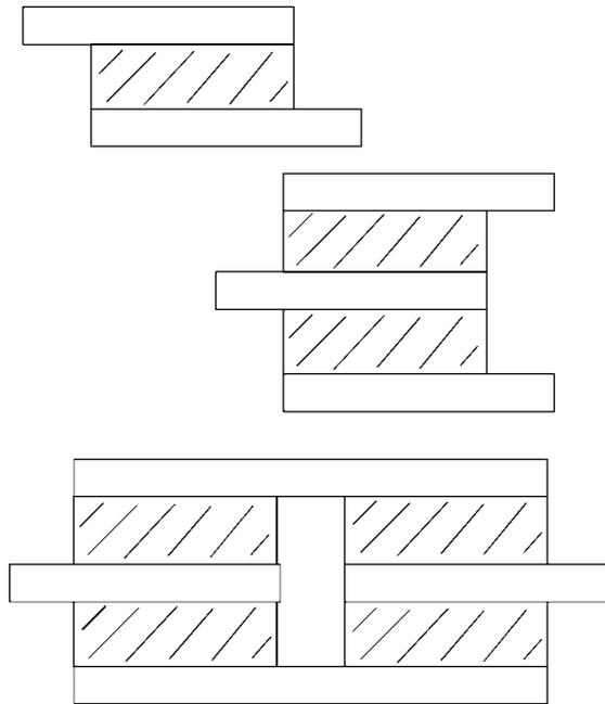
Figure 8.3 Lap and sandwich shear test pieces
