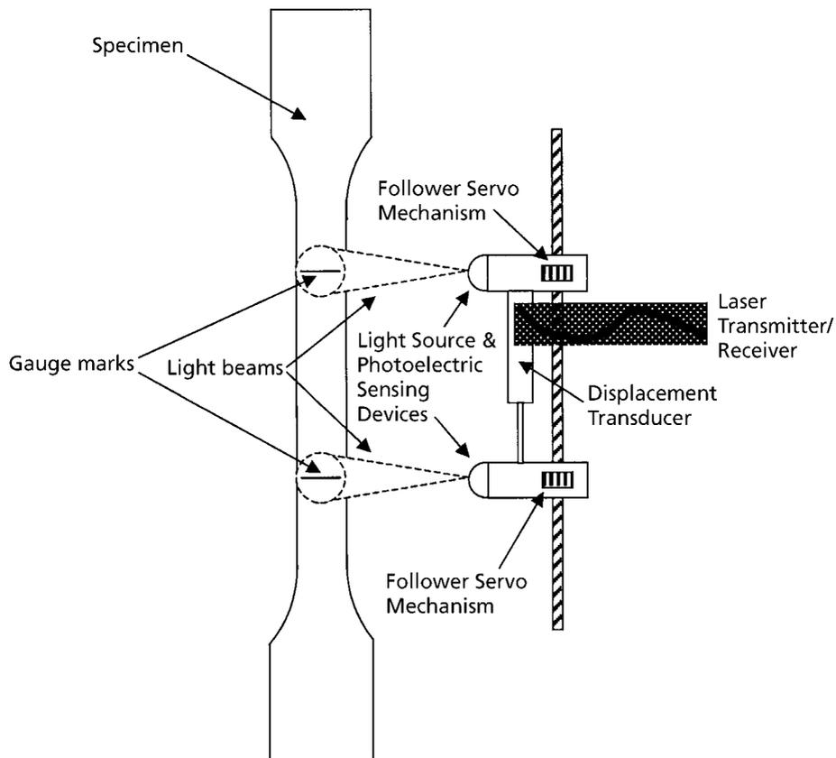
**Figure 6.17** Optical extensometer
