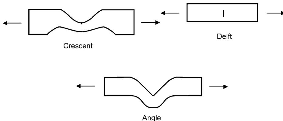
**Figure 11.1** Tear test piece geometries
