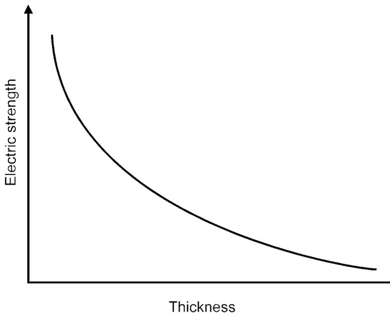
**Figure 1.3** Electric strength as a function of thickness
