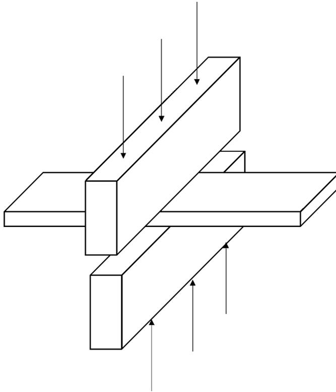
**Figure 7.2** Plain strain compression test
