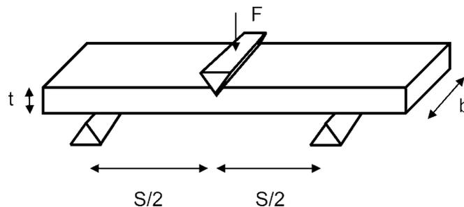
**Figure 1.2** General arrangement for flexural strength measurement
