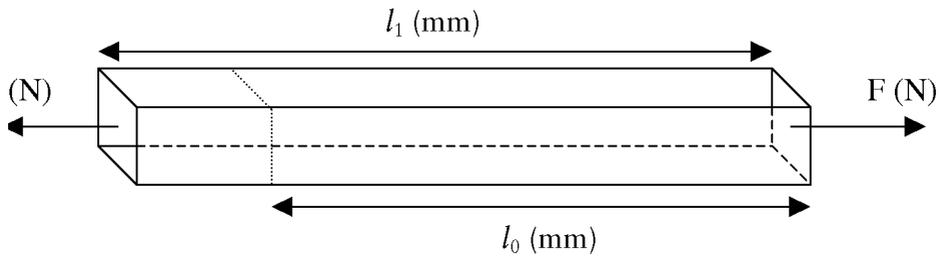
**Figure 6.3** Tensile strain generated in a rectangular bar
