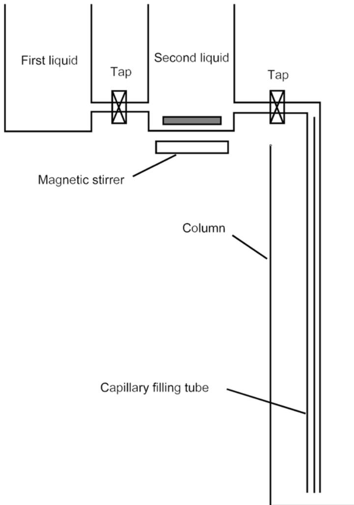
**Figure 4.1** Preparation of a density column
