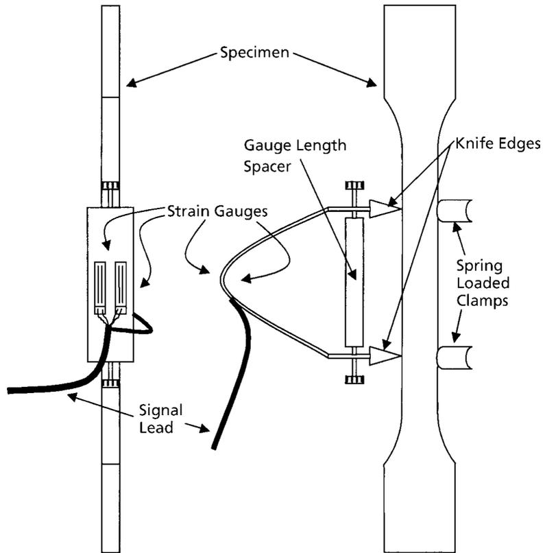
Figure 6.16 Schematic of a clip on strain gauge extensometer
