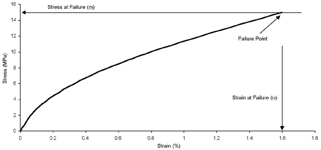
Figure 6.8 Typical stress *versus* strain characteristic of a brittle thermoplastic
