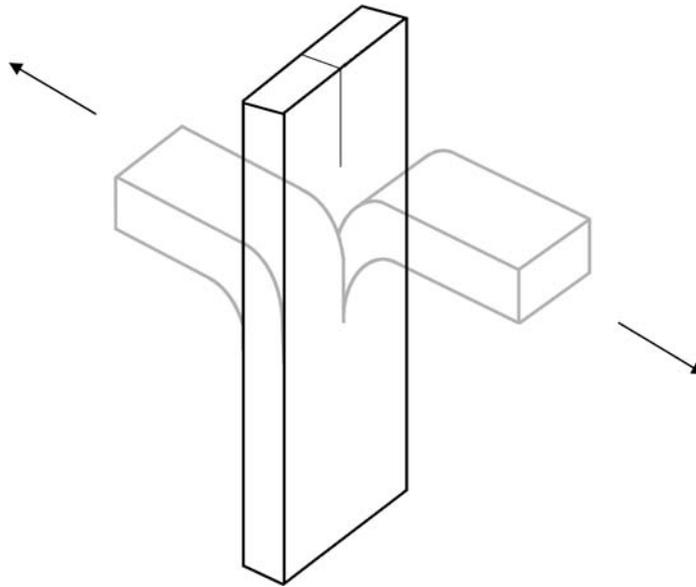
Figure 11.2 Trouser tear test piece
