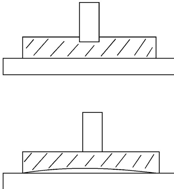
**Figure 4.3** Possible errors in thickness measurement
