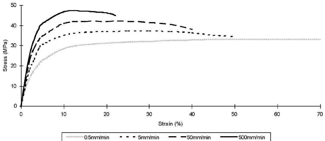
Figure 6.11 HDPE tensile stress *versus* strain curves at 23 °C and increasing strain rates
