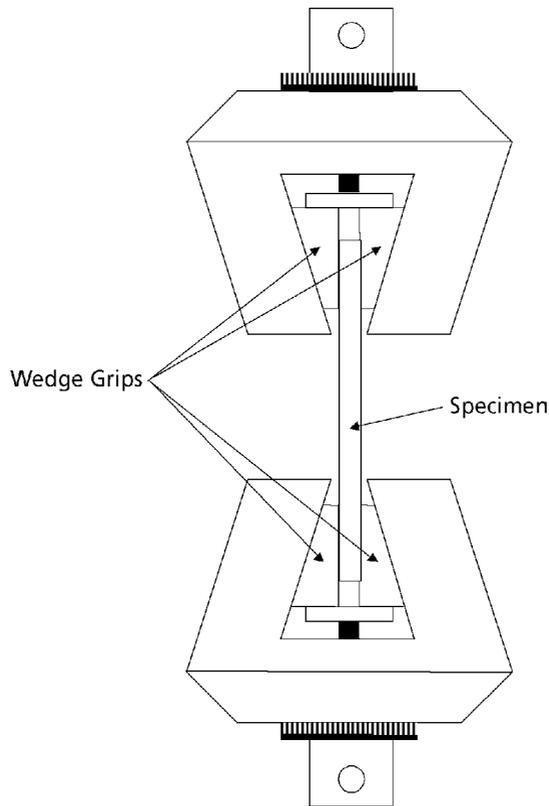
**Figure 6.15** Typical wedge grip assembly
