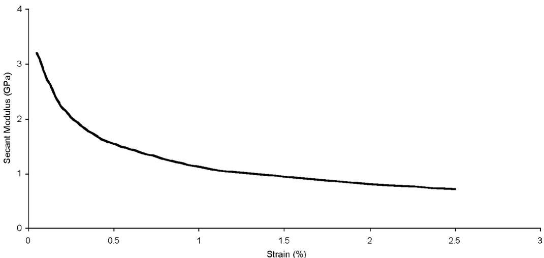
**Figure 6.10** Secant modulus *versus* strain for a typical non-linear thermoplastic
