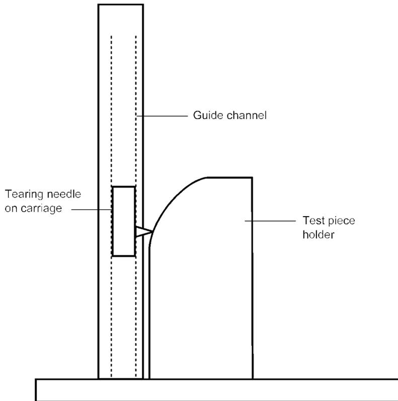
Figure 11.5 ASTM puncture propagation
