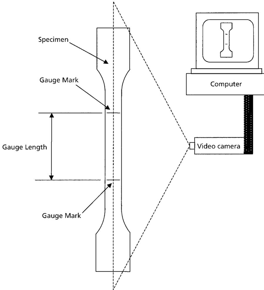
**Figure 6.19** Video extensometer
