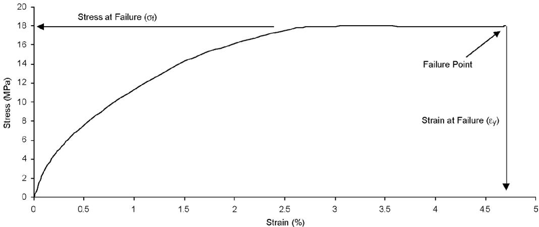
**Figure 6.7** Typical non-linear stress *versus* strain characteristic of a tough thermoplastic showing no drop in stress at yield
