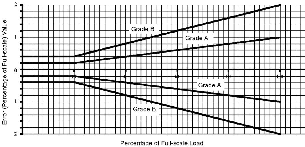
Figure 6.12 Machine accuracy gradings
