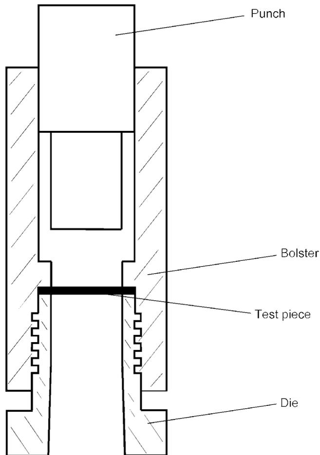
**Figure 8.4** Arrangement for punch shear
