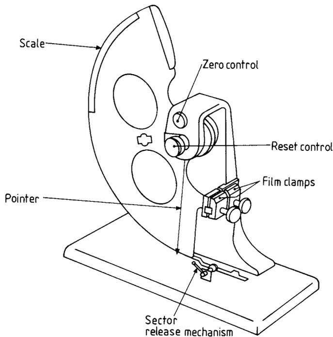
**Figure 11.4** Elmendorf tear tester
