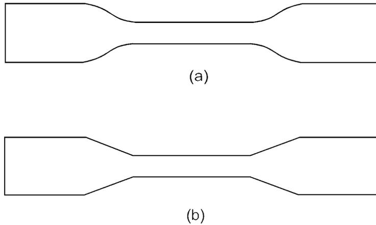
**Figure 1.1** Possible shapes for tensile test pieces
