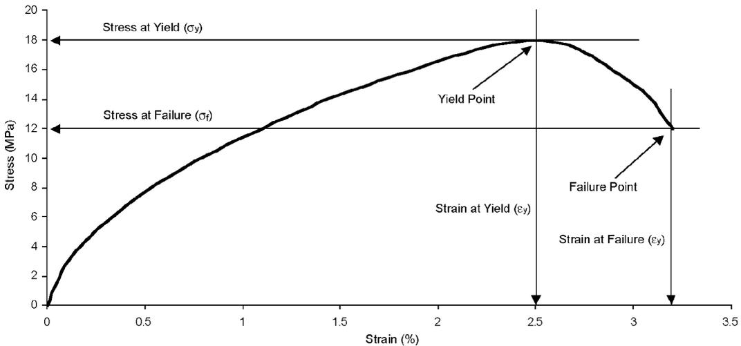
Figure 6.5 Typical non-linear stress *versus* strain characteristic for a material with a yield stress greater than the failure stress
