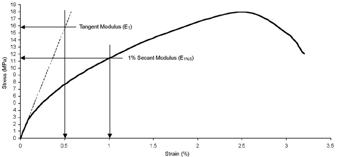
Figure 6.9 Determination of the modulus of a typical non-linear thermoplastic
