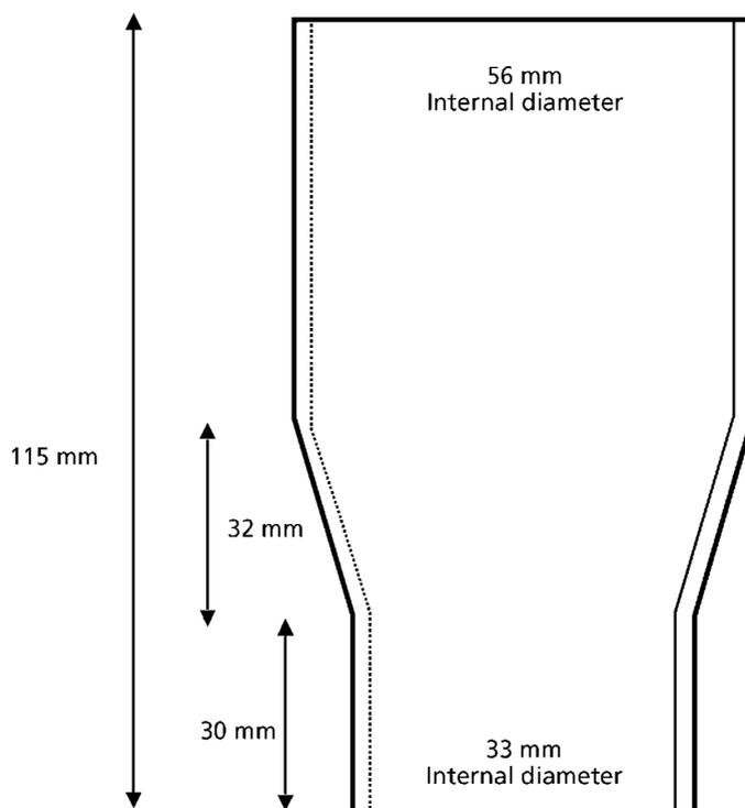
**Figure 4.2** Form of funnel for apparent density
