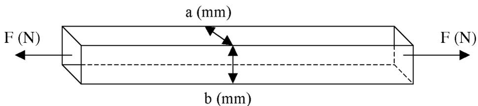
**Figure 6.1** Tensile stress generated in a rectangular bar
