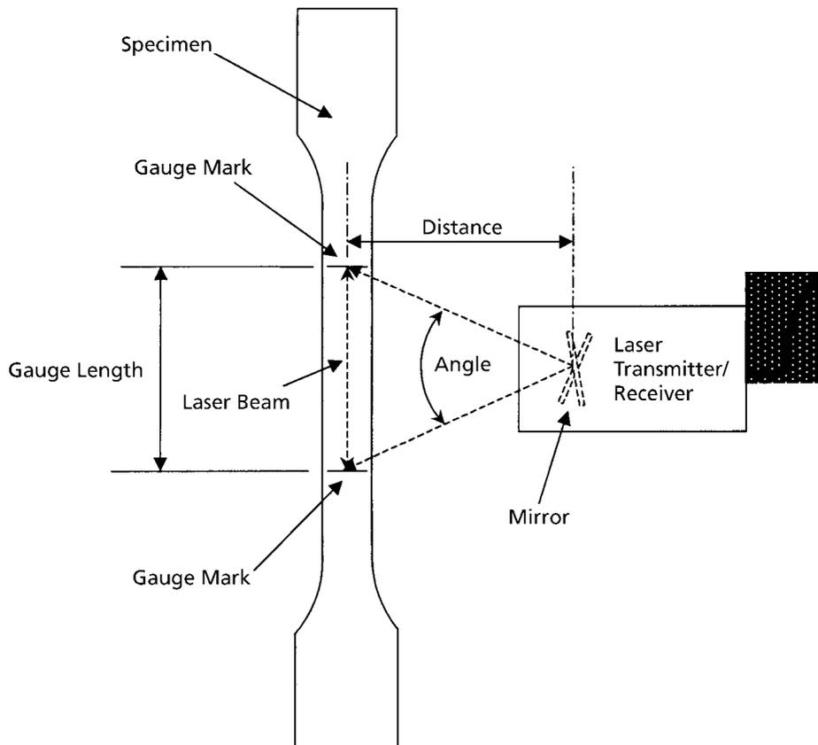
Figure 6.18 Laser extensometer
