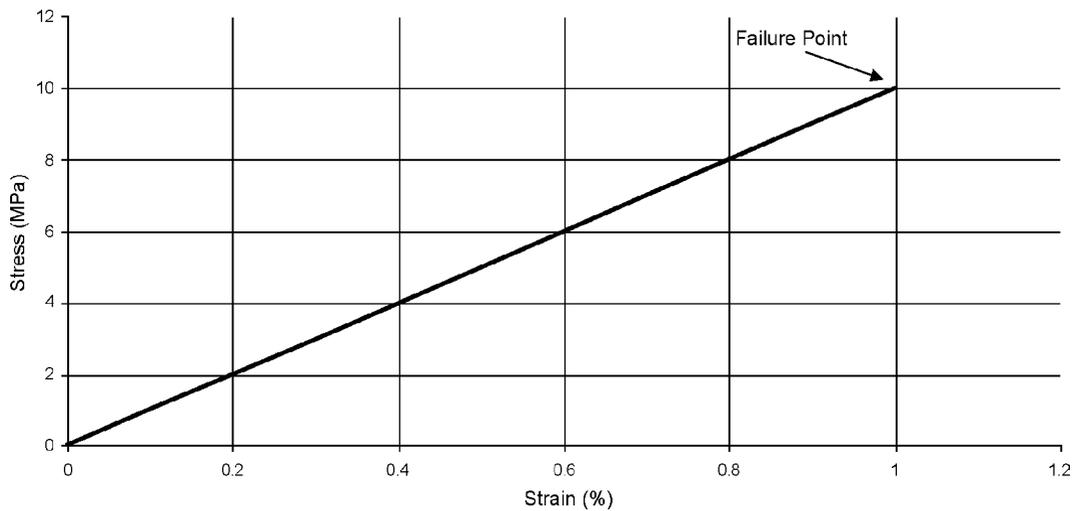
**Figure 6.4** Typical stress *versus* strain characteristic for a perfectly elastic solid
