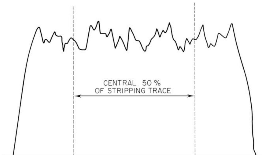
**Figure 11.3** Tear or peel adhesion trace
