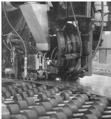
Automated welding system for the production of door inner blanks. Source: TWB Company.
