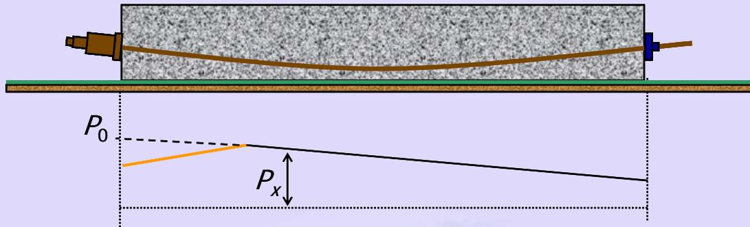
**Figure 2-2.4** Variation of prestressing force after anchorage slip
