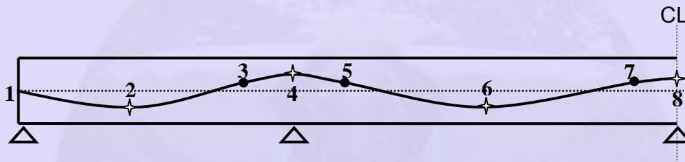
The following properties of parabolas are used. For segment 1-2, the parabola in the sketch below is used.
