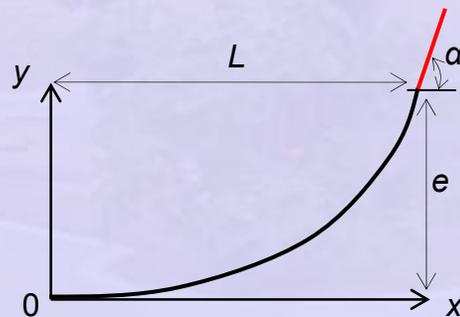
The change in slope from the origin to the end of the parabola is same as the slope at the end which is  $\alpha = 2e/L$ , where
