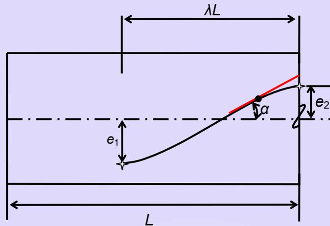
For the two parabolic segments joined at the inflection point as shown in the sketch above, the slope at the inflection point  $\alpha = 2(e_1 + e_2)/\lambda L$ .
