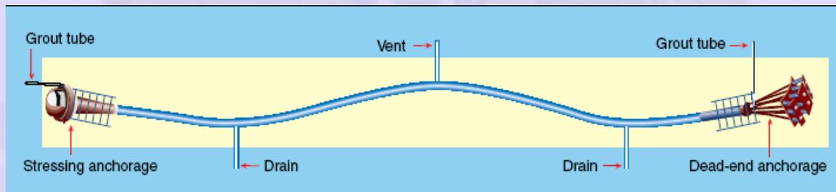
**Figure 2-2.1** A typical continuous post-tensioned member
