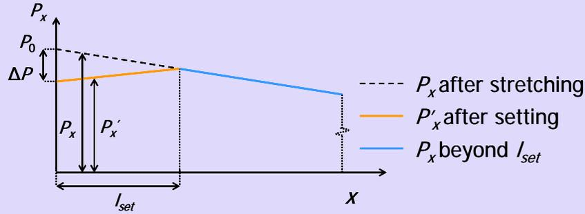
**Figure 2-2.5** Force variation diagram near the stretching end
