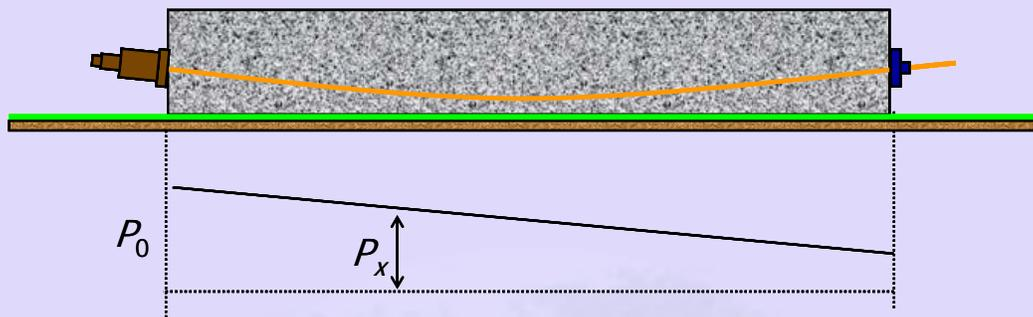
**Figure 2-2.3** Variation of prestressing force after stretching
