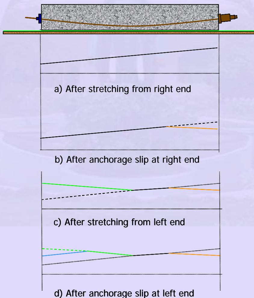
**Figure 2-2.6** Force variation diagrams for stretching in stages
