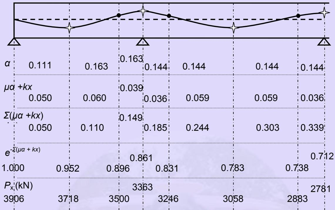
The force variation diagram before anchorage can be plotted with the above values of  $P_x$ . A linear variation of the force can be assumed for each segment. Since the stretching is done at both the ends simultaneously, the diagram is symmetric about the central line.
