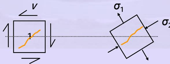
**Figure 5-1.3** Inclination of crack at the level of neutral axis
