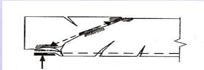
**Figure 5-1.13** Arch rib failure
