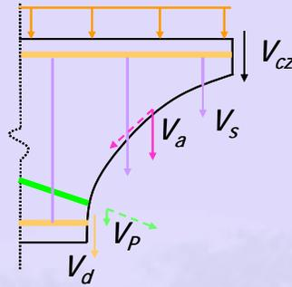
**Figure 5-1.8** Internal forces at a flexure shear crack
