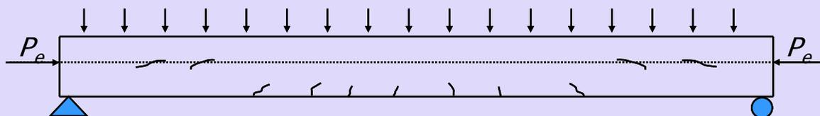
**Figure 5-1.16** Formation of cracks in a prestressed beam
