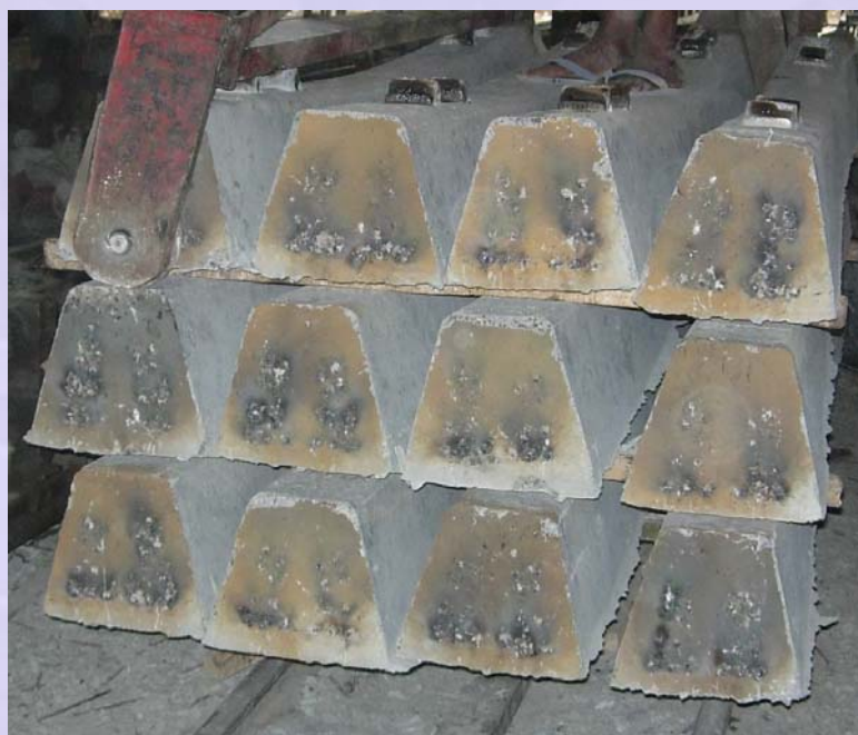
Figure 7-1.1 End of pre-tensioned railway sleepers
