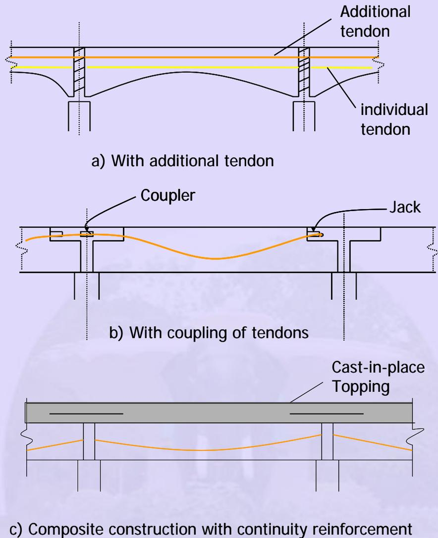
**Figure 8-3.6** Partially continuous beams
