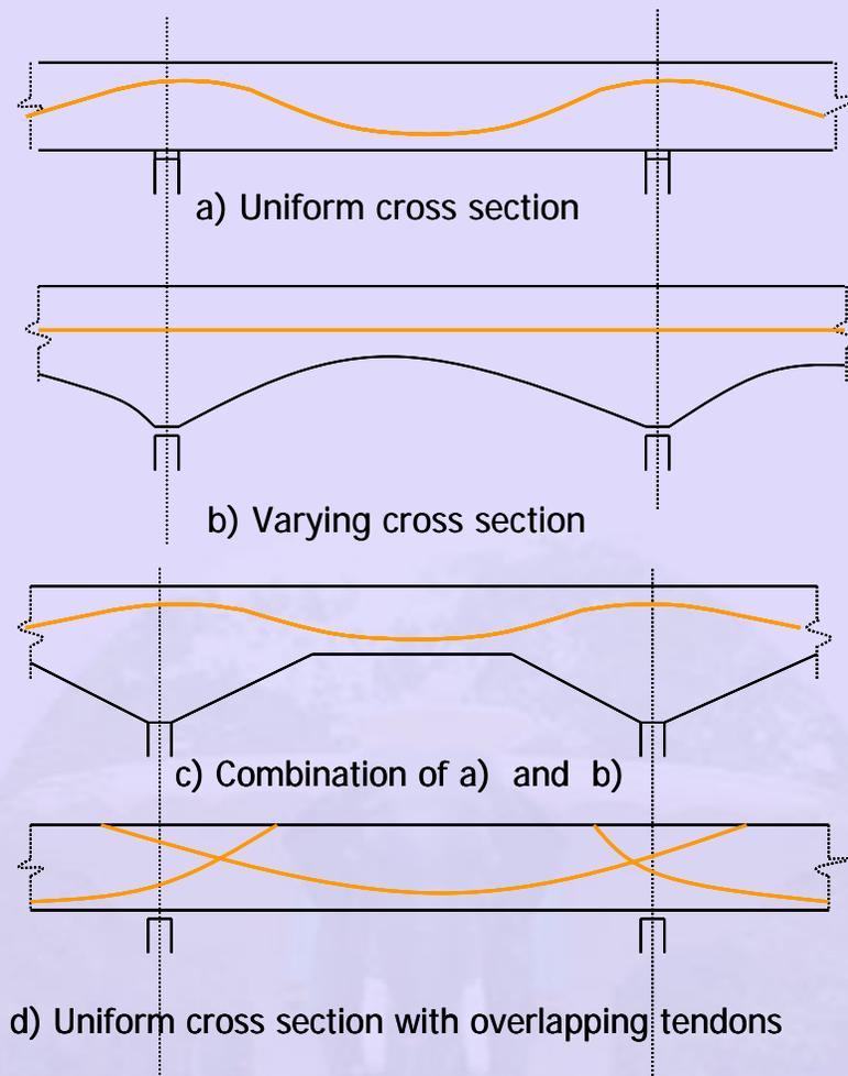
**Figure 8-3.5** Profiles of CGS for continuous beams
