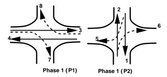
Figure 41:2: Two phase signal
