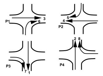
Figure 41:5: Third possible way of providing a four-phase signal
