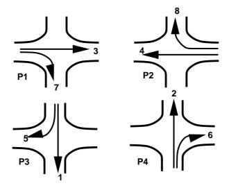
Figure 41:3: One way of providing four phase signals
