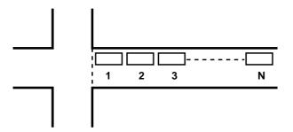
Figure 41:6: Group of vehicles at a signalized intersection waiting for green signal
