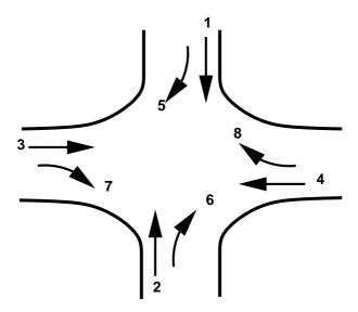
Figure 41:1: Four legged intersection
