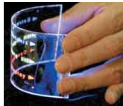
Colors are bright in a flexible display made of a hybrid of inorganic and organic LEDs by a group at the University of Cincinnati.
