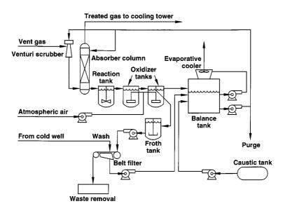
FIGURE 7.8.1 Typical equipment used in the Stretford process for hydrogen sulfide abatement at The Geysers geothermal field. (Based on the diagram of Henderson, J.M. and Dorighi, G.P., *Geotherm. Resour. Counc. Trans.*, 13, 593–595, 1989.)
