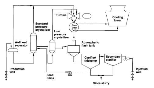
**FIGURE 7.8.3** The flow stream for removal of solids from the vapor and brine in typical power plants in the Salton Sea geothermal field. (Modified from the diagram of Signorotti, V. and Hunter, C.C., *Geotherm. Resour. Counc. Bull.*, 21(9), 277–288, 1992).
