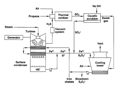
FIGURE 7.8.2 Equipment used in the incineration process for hydrogen sulfide abatement at The Geysers geothermal field. (Based on the diagram of Bedell, S.A. and Hammond, C.A., *Geotherm. Resour. Counc. Bull.*, 16(8), 3–6, 1987.)
