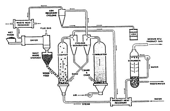
FIGURE 7.4.2. A diagram illustrating the Battelle Biomass Indirect Gasification System.
