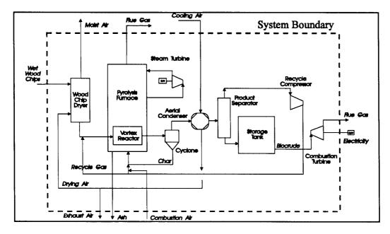
FIGURE 7.4.3. A diagram illustrating the biomass fast pyrolysis process for biocrude oil production.
