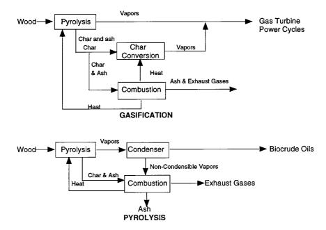
**FIGURE 7.4.1.** A diagram illustrating biomass gasification and pyrolysis processes. (From U.S. Department of Energy, *Electricity from Biomass: A Development Strategy.* DOE/CH10093-152, DE92010590. Washington, D.C., 1992.)
