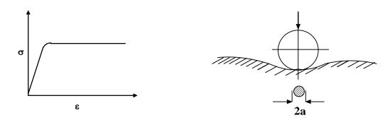
**1.2.6.1F**- Stress-strain diagram of an elastic-perfectly plastic material and the plastic indentation.
