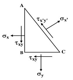
2.2.5.2F- Stresses on an isolated triangular element
