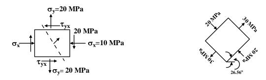
**2.2.6.2F-** Orientation of the loaded element in the left to show the principal stresses.
