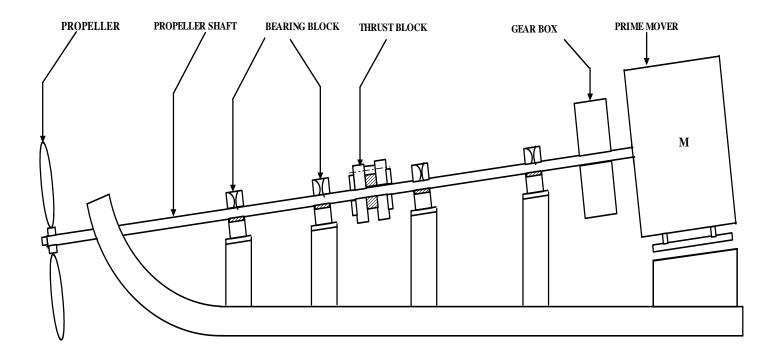
2.2.4.2F- A schematic diagram of a typical marine propulsion shafting
