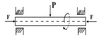
**2.2.4.1F-** A simply supported shaft subjected to axial force bending moment and torsion.
