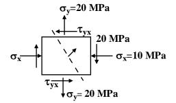
**2.2.6.1F-** A 2-D element with normal and shear stresses.
