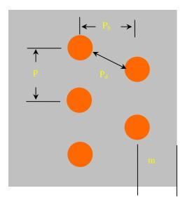
Figure 10.17: Important design parameters of riveted joint
