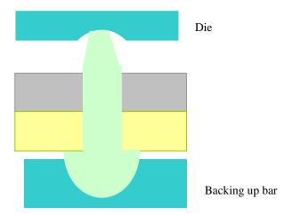
Figure 10.1.2: Riveting operation
