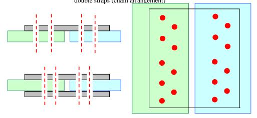
Figure 10.1.6(c): Double riveted butt joint with single and double straps (zig-zag arrangement)
