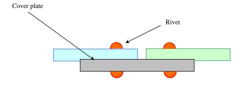
Figure 10.1.5: Butt joint with single strap.
