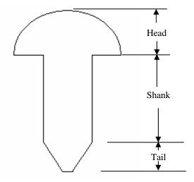
Figure 10.1.2: Rivet and its parts
