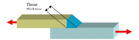
Figure 10.4.2: Design of a single transverse fillet
