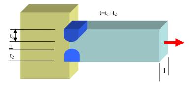
Figure 10.4.1: Design of a butt joint
