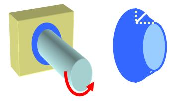
Figure 10.4.5: Design of a fillet weld for torsion
