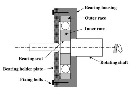
Fig. 14.2.2 A typical arrangement for housing a bearing
