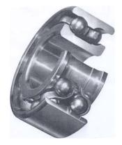
Double Row Angular Contact Bearing, shown in Fig.14.2.4, has two rows of balls. Axial displacement of the shaft can be kept very small even for axial loads of varying magnitude.
