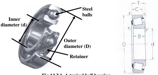
Fig.14.2.1 A typical ball bearing
