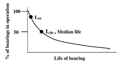
Fig. 14.2.9 Definition of life of rolling contact bearing
