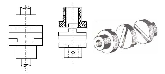
5.1.2.2.1.1F- A schematic diagram of an Oldham coupling
