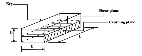
5.1.2.1.1.2F- Shear and crushing planes in the key.
