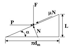
**6.1.2.3 F-** Forces at the contact surface for raising the load.
