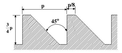
6.1.1.4F – Some details of a Buttress thread form
