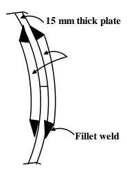
9.1.2.1F- Longitudinal welded joint with cover plates.
