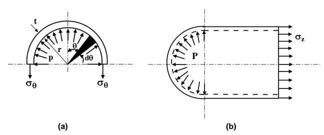
9.1.1.2F- (a) Circumferential stress in a thin cylinder (b) Longitudinal stress in a thin cylinder
