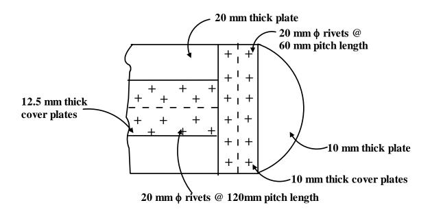
9.1.2.4F- General riveting arrangement of the pressure vessel.
