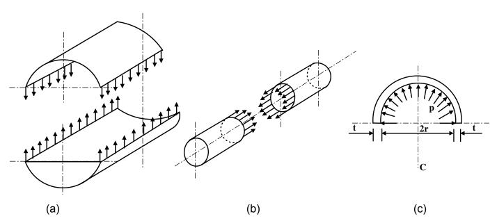
9.1.1.1F- (a) Circumferential stress (b) Longitudinal stress and (c) Radial stress developed in thin cylinders.
