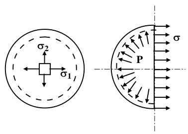
9.1.1.3 F- Stresses in a spherical shell
