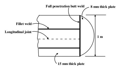
9.1.2.2F- The welding arrangement of the joint.
