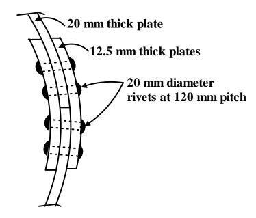
9.1.2.3F- A longitudinal joint with two cover plates
