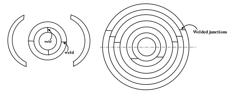
9.2.2.4F- Method of construction of multilayered cylinder
