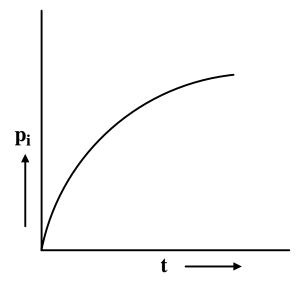
9.2.2.1F- A schematic variation of wall thickness with the internal pressure in a thick walled cylinder.
