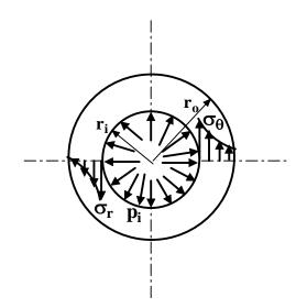
9.2.1.3F- Radial and circumferential stress distribution within the cylinder wall when only internal pressure acts.
