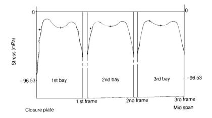
Figure 6.12 Longitudinal stress of the innermost fibre at 0.6895 MPa (100 psi), Model No. 2.
