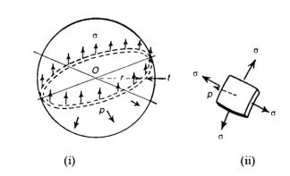
Figure 6.6 Membrane stresses in a thin spherical shell under internal pressure.
