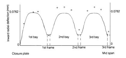
Figure 6.9 Deflection of longitudinal generator at 0.6895 MPa (100 psi), Model No. 2.
