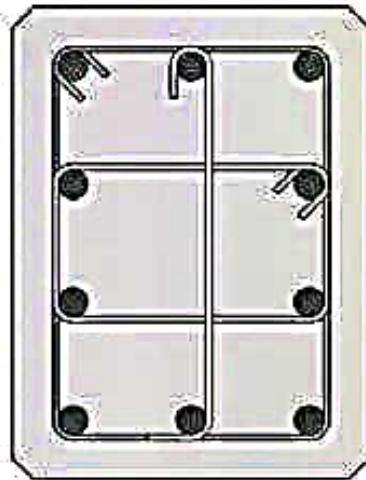
(d) Tie arrangement in a rectangular column with 10 longitudinal bars and a set of three ties
