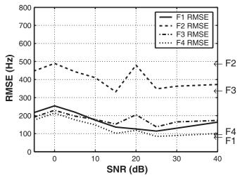
Fig. 7. Mean RMSE (in Hz) over 25 trials as a function of SNR (in dB) for a synthesized male speaker saying "Once upon a midnight dreary, while I pondered weak and weary, over many a..." in the presence of background babble. The arrows indicate the standard deviation of the actual formant frequency values (in Hz).
