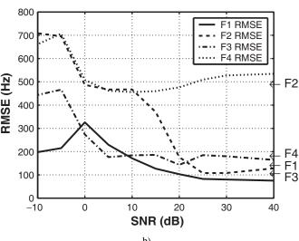
Fig. 5. Formant tracking results for a synthesized female speaker saying "Five women played basketball" in the presence of background white Gaussian noise. a) Spectrogram, estimated (solid lines) and actual (dotted lines) formant frequencies, and voicing decision (dashed line) at an SNR of 20 dB. b) Mean RMSE (in Hz) over 25 trials as a function of SNR (in dB). The arrows indicate the standard deviations of the actual formant frequency values (in Hz).
