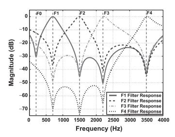
Fig. 2. The magnitude-frequency response of the four formant filters at a particular time when the pitch (F0) is set to 200 Hz, the first formant frequency (F1) is set to 700 Hz, the second formant frequency (F2) is set to 1500 Hz, the third formant frequency (F3) is set to 2200 Hz and the fourth formant frequency (F4) is set to 3500 Hz. Each formant filter acts as an adaptive bandpass filter, spectrally isolating the four formants.
