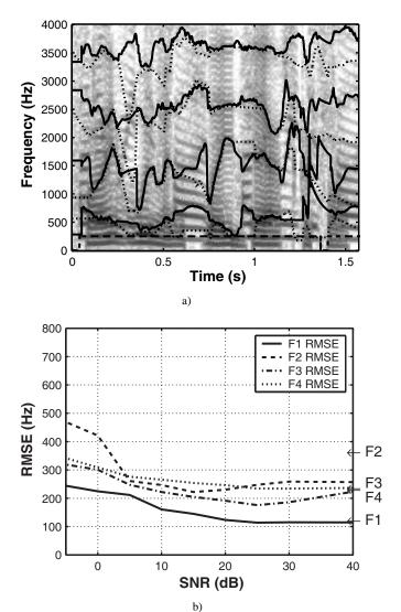
Fig. 6. Formant tracking results for a synthesized male speaker saying "Five women played basketball" in the presence of a single recorded (TIMIT) female speaker. a) Spectrogram, estimated (solid lines) and actual (dotted lines) formant frequencies, and voicing decision (dashed line)at an SNR of 5 dB. b) Mean RMSE (in Hz) over 25 trials as a function of SNR (in dB). The arrows indicate the standard deviation of the actual formant frequency values (in Hz).
