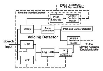
Fig. 4. Block diagram of the voicing detector designed to identify voiced segments of speech.
