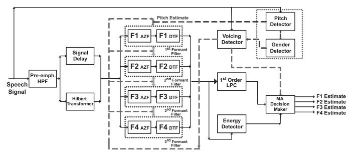
Fig. 1. Block diagram of the formant tracker. The formant tracker relies on an adaptive filterbank to separate each formant frequency region prior to spectral estimation.
