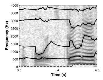
Fig. 8. Spectrogram, formant frequency estimates (solid lines) and gender decision (dashed line) for a transition between a male and a female speaker (at  $t \approx 4.1 \, \mathrm{s}$ ) in the presence of AWGN at an SNR of 25 dB. Where the dashed line is low the gender detector has determined that the speaker is male, and where the dashed line is high it has decided that a female has begun speaking.
