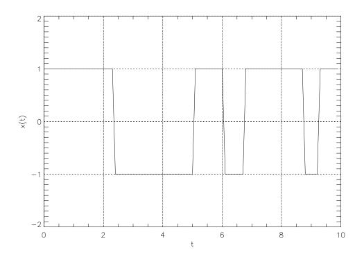
Figure 7.4: An example of a telegraph signal. The zero cossings are described by a Poisson process, with an average rate of  $\lambda = 1$  per second.
