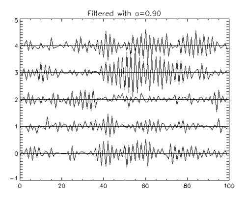
Figure 7.6: Ensemble of outputs of digital filter with white noise input and filter equation y[n] = x[n] + 0.9y[n-1], which represents a low-pass digital filter.
