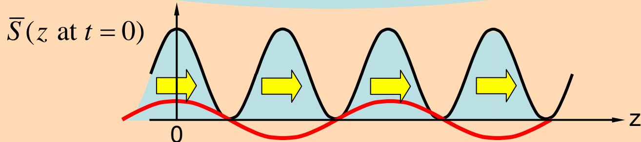
$$\bar{S} = \hat{z} \frac{E_0^2}{\eta_0} \cos^2(\omega t - kz) \Rightarrow \langle \bar{S} \rangle = \hat{z} \frac{1}{2} \frac{E_0^2}{\eta_0} = I(\theta, \phi, r) \text{ [W/m}^2\text{]}$$
