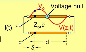
Cannot excite  $TEM_m$  modes by driving current into voltage nulls! (Or by voltage sources in series at current nulls).  $P_{in}(t) = 0$  in both cases.
