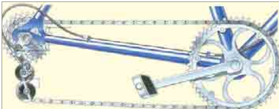
Sports bicycle gear and chain drive mechanism
