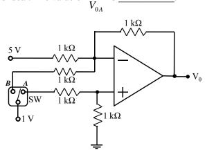
Q.13 In the bistable circuit shown, the ideal opamp has saturation levels of  $\pm 5$  V. The value of  $R_1$  (in k $\Omega$ ) that gives a hysteresis width of 500 mV is \_\_\_\_\_.
