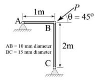
Q.21 The plane frame shown is analyzed by neglecting axial and shear deformations. The horizontal displacement of **joint B** is
